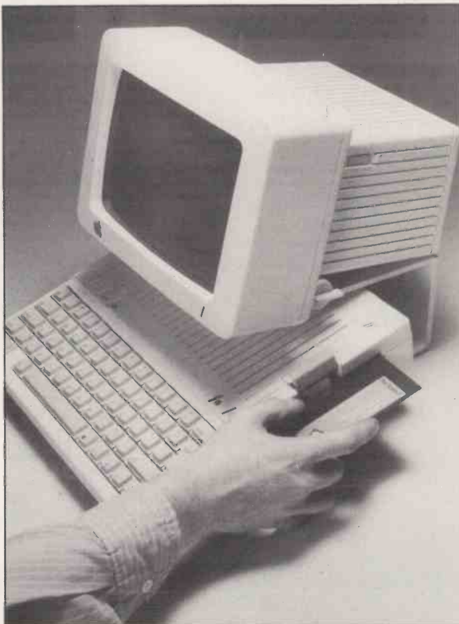
A slot on the right-hand side of the IIc provides access to the half-height 5.25in. minifloppy disc-drive unit.
